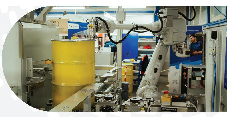
This project is intended to automate the characterization of radioactive waste at Nuclear Plants, and make the characterization process more effective, safer for operators and more reliable due to process repeability. The aim of the project was design, software development, manufacturing, installation on site and commissioning of two different systems.
